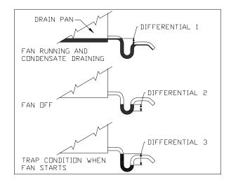
FIGURE 7 - CONDENSATE DRAIN TRAP
